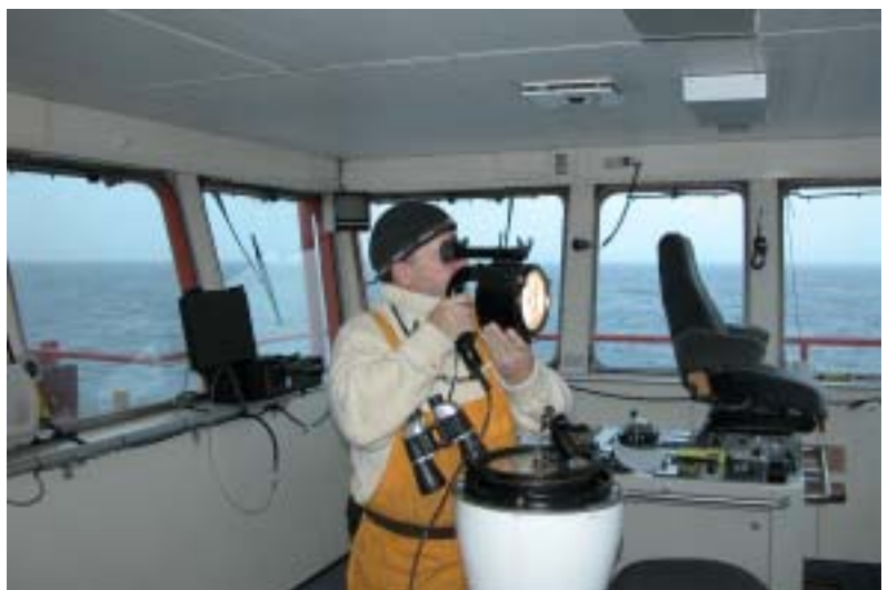
Signalling the unidentified vessel using an Aldis Lamp with International Morse Code signals.
